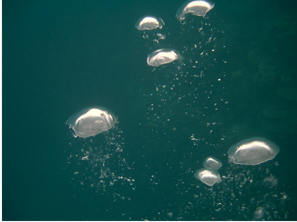
FIGURE 5 – rising bubbles, those are too large to apply Hadamard-Rybczynski theory. Those are Taylor bubbles which are inertial, so that drag is scaled by \rho U_0^2 L^2 .
