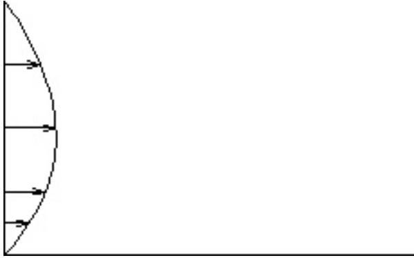
Figure 2: Basic Poiseuille profile, [click on the Image] to see the effect of aspiration
