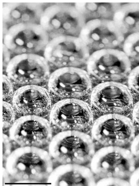
12 A few seconds after pouring and after collapse of foamy head, surface of flute is covered with layer of quite mono disperse millimetric bubbles, where bubbles arrange themselves in approximate hexagonal pattern, strikingly resembling those in beeswax (bar is 1 mm)
