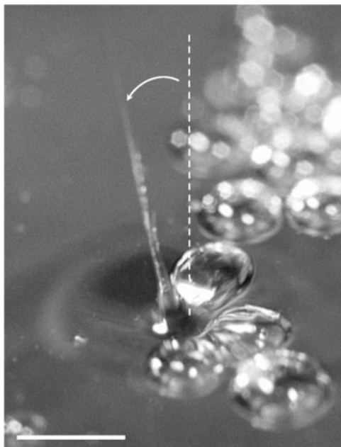
20 Close-up on tilted Worthington jet (frozen through high speed photography) as neighbouring bubbles' symmetry is broken around collapsing one (bar is 1 mm)
