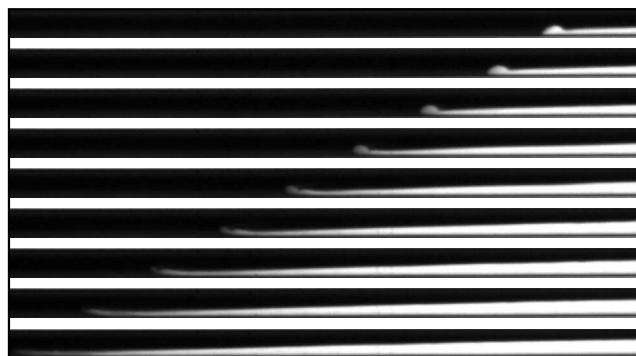
FIG. 4. Sequence of images showing the initial bump shape spread out by the Poiseuille velocity gradient. This sequence is obtained for \theta=87^\circ , At=10^{-2} , and \mu=10^{-3} Pa s, and the mean flow ( V_0=77.4 mm s ^{-1} ) is imposed after the first image (top one). The field of view is 452 \times 20 mm ^2 and taken a few centimeters below the gate valve. The sequence starts 7 s after opening the gate valve and the time interval between images is \Delta t=0.5 s.
