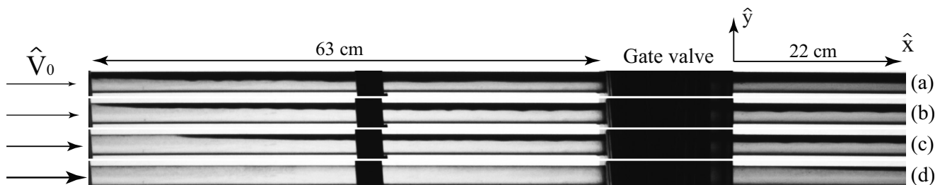
FIG. 3. Four snapshots of video images taken at different mean flow rates and illustrating the different regimes. The heavy transparent fluid flows downward under the combined effects of buoyancy ( \Delta\rho ) and pressure gradient ( \hat{V}_0 ). The light black fluid has different behaviors (flows upward or downward) depending on the control parameters values. These images were obtained at \beta=85^\circ , At=10^{-2} , and \hat{\mu}=10^{-3} Pa·s. The mean flow velocities were: (a) \hat{V}_0=29 mm·s ^{-1} , (b) \hat{V}_0=38 mm·s ^{-1} , (c) \hat{V}_0=42 mm·s ^{-1} , and (d) \hat{V}_0=61 mm·s ^{-1} . The field of view is 1015 \times 20 mm, and contains the gate valve (wide black stripe) and a pipe support (thin black stripe). The images are taken at: (a) 150 s, (b) 290 s, (c) 365 s, and (d) 75 s after opening the valve.
