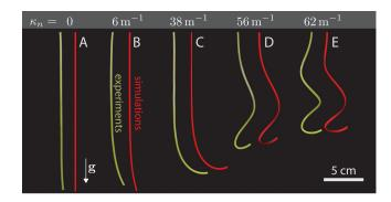
FIG. 1 (color online). Equilibrium shapes of rods suspended under their own weight: comparison of experiments and simulations. The natural curvature  $\kappa_n$  is varied, while the length L=20 cm, radius r=1.55 mm, elasticity parameters (E=1290 kPa,  $\nu=0.5$ ), and volumetric mass  $\rho=1200$  kg/m³ are kept constant.
