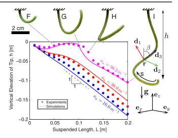
FIG. 2 (color online). Vertical elevation of the tip h versus arc length of the rod L, for three different natural curvatures  $\kappa_n = (16.6, 38.0, 56.2) \text{ m}^{-1}$ : experiments (circles) and simulations (solid lines). For  $\kappa_n = 56.2 \text{ m}^{-1}$ , the configurations F and G are planar while the configurations H and I are nonplanar.
