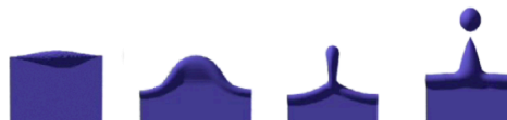
Fig. 9.8. A possible mechanism for droplet formation, involving an initially deformed bulging end rim.
