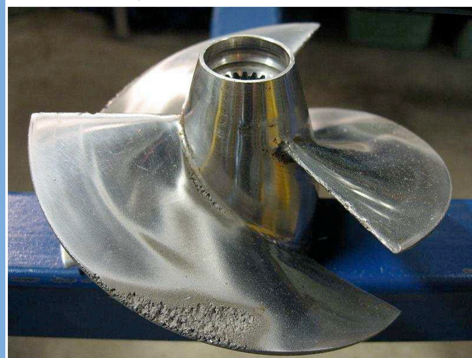
Figure: Cavitation damage evident on the propeller. Concentrated damage on the outer edge of the propeller where the speed of the blade is high.
