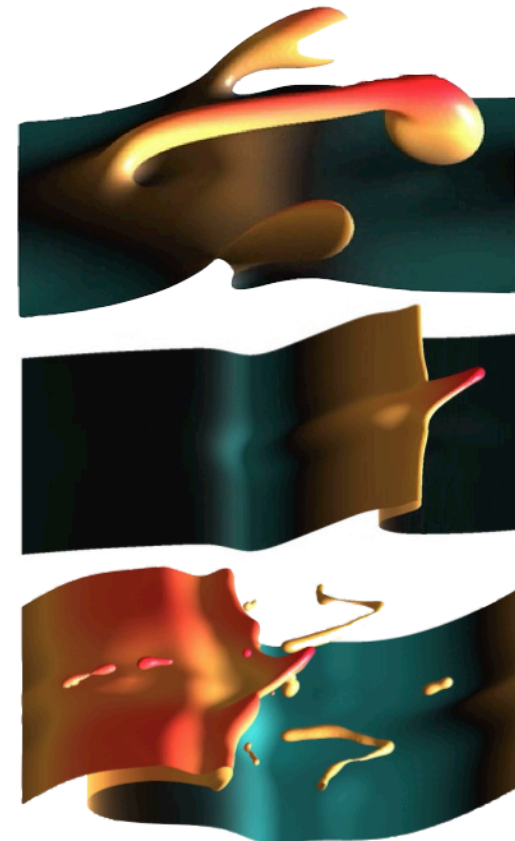
FIGURE 2. Jet emerging from 0.25 in. diameter nozzle into stagnant air. Jet velocity = 83 ft/s.
