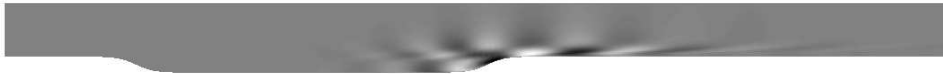
Figure 3: Overview of the real part of the u -component of the most unstable eigenmode.
