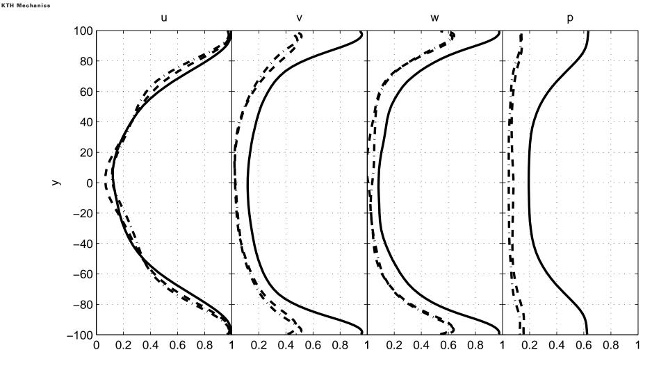
Plant / estimator correlation of velocity and pressure in wall-normal direction.
