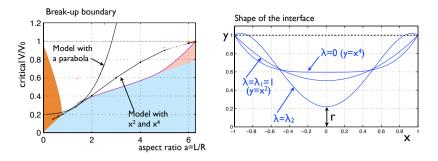
Figure 3.3: Left: Comparison of the breakup boundary with that predicted by the one degree of freedom model and the two degrees of freedom model. Right: Shapes of the liquid bridge with different values of the second degree of freedom  $\lambda$ .
