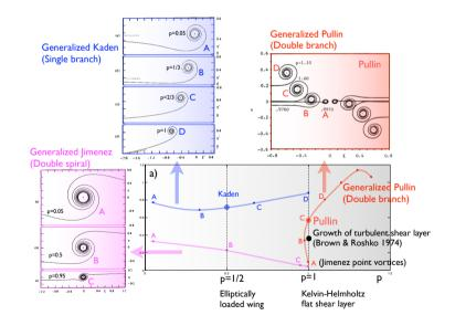
Figure 4.8: General families of self-similar solutions on a vortex sheet of varying intensity.
