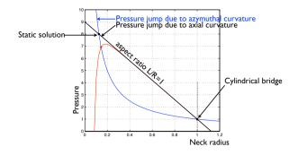
Figure 3.2: The graphical mechanism that can be used as an analogue to the physical mechanism for breakup of the static liquid bridge.
