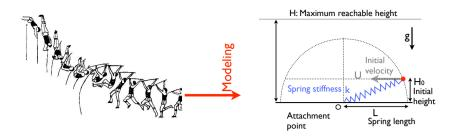
Figure 1.8: Modelling of the pole vault. Left: image from [Ganslen, 1961].
