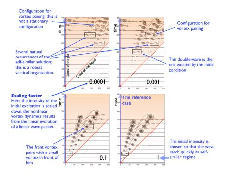
Figure 4.13: Impulse response of the shear-layer, with scaling of the initial intensity.
