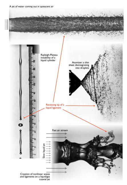
Figure 4.1: Images of creating droplets from a liquid body: atomization. All images come from [VanDyke, 1982] except the coaxial jet which comes from [Marmottant and Villermaux, 2004].
