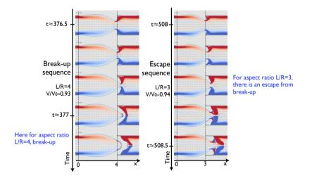
Figure 2.9: Final breakup of the capillary Venturi, and escape from this breakup.
