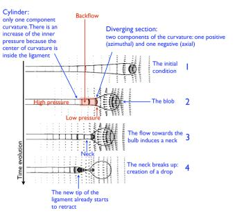
Figure 2.5: The end-pinching mechanism for creation of the neck. Image adapted from [Stone and Leal, 1989].
