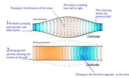
Figure 2.1: Comparison between the wall-deformation peristalsis and the blowing and suction pumping.
