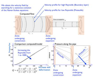
Figure 2.3: Quantitative validation of the piecewise-continuous channel for peristalsis.
