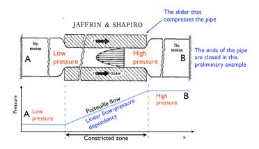
Figure 2.2: Sketch for the pumping mechanism of peristalsis. Image adapted from [Jaffrin and Shapiro, 1971].
