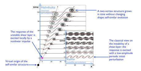
Figure 4.2: Helmholtz' spiral and the Kelvin periodic row of vortices. These are the response of the unstable shear layer to two different types of excitations: periodic and low amplitude, or localized and large amplitude.
