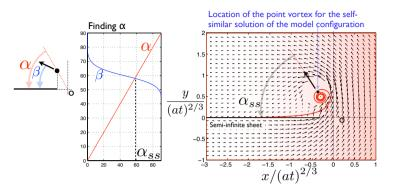
Figure 4.7: Results of the point-vortex model for the rollup of the wingtip vortex.
