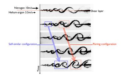
Figure 4.14: A shear layer at pressure 8 atmospheres and Reynolds 850,000. Image from [VanDyke, 1982].
