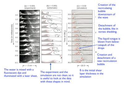
Figure 4.11: Experiments and numerical simulation for the catapult mechanism of droplets by the self-similar wave.
