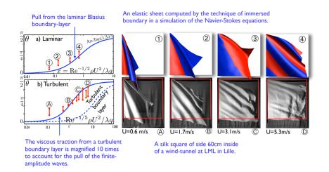
Figure 1.5: Numerical simulation of a flag flowing in the Navier-Stokes equations, and experiment with square of silk in LML's wind tunnel.
