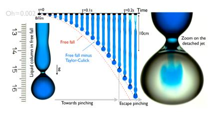
Figure 2.6: Free-falling liquid column experiment showing the escape of pinch-off.
