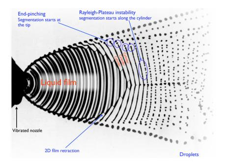
Figure 2.4: The ways to make drops from liquid cylinders exemplified on a vibrated film atomizer. Image adapted from [VanDyke, 1982].
