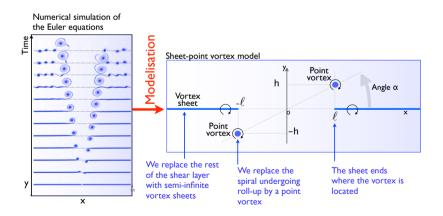
Figure 4.5: A vortex sheet-point vortex model for the self-similar structure.
