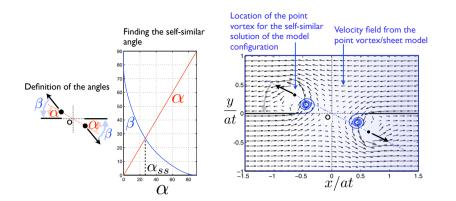
Figure 4.6: Results of the point-vortex model for the impulse response of the shear-layer.
