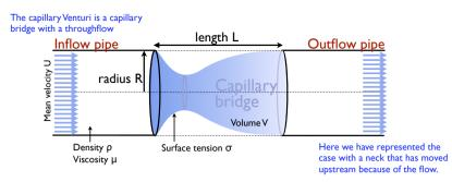
Figure 2.7: Sketch of the capillary Venturi.
