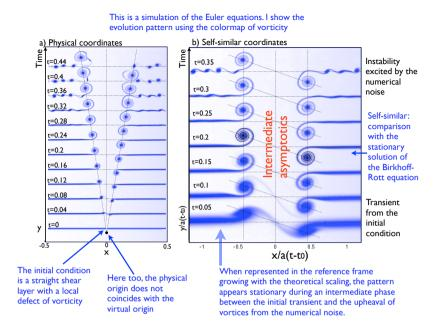
Figure 4.4: Rescaling of the frame to show the intermediate asymptotics of the self-similar response to a localized excitation of the shear layer.
