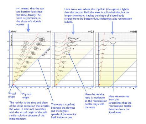
Figure 4.3: The self-similar response of the shear layer to a local excitation for three different values of the density ratio r.
