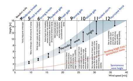
Figure 4.10: Comparison of the size of the self-similar structure and the shedding length of droplets with indications of the Beaufort wind scale.
