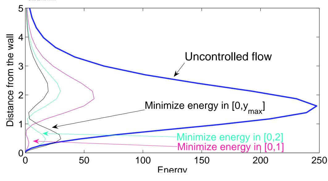
The controller seeks to eject the disturbance out of the B.L.
