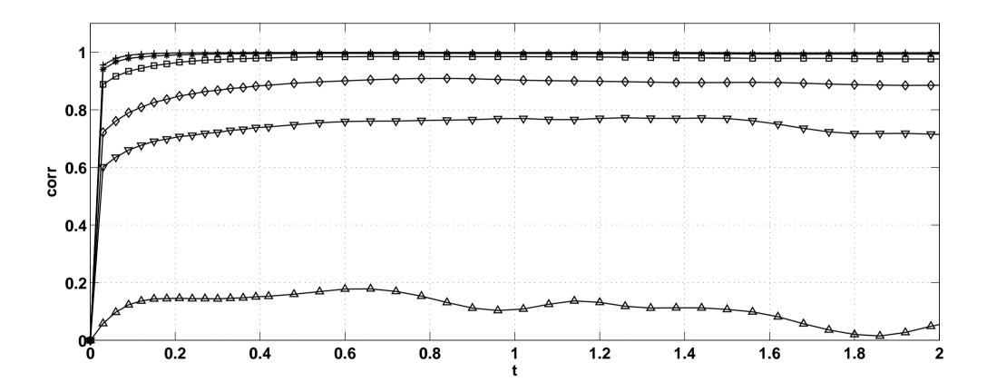
Estimation transient for the streamwise velocity u at  $y^+ = 1.5$ ,  $y^+ = 5.5$ ,  $y^+ = 9.7$ ,  $y^+ = 19.8$ ,  $y^+ = 31.5$ , and along the channel centreline
