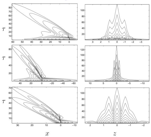
The transfer function in time, integrated in the streamwise direction (left column) and spanwise direction (right column) for the three measurement, streamwise skin friction (top), spanwise skin friction (middle) and pressure (bottom).
