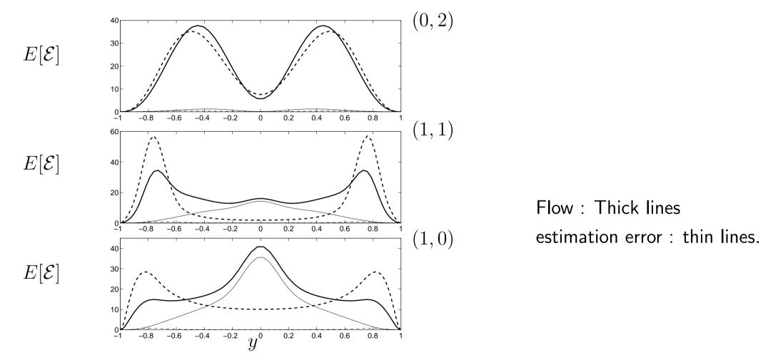
Estimation performance for disturbances in all the domain (solid lines) and close to the walls (dashed lines).
