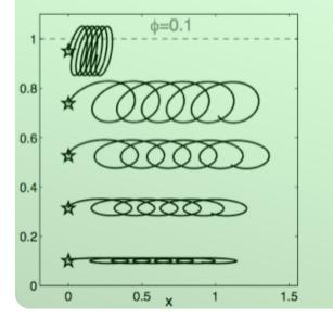
For **blowing and suction**, the particles' forward motion takes place close to the walls, where viscosity slows down the flow.
