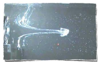
Jet generated by an ultrasonic beam
