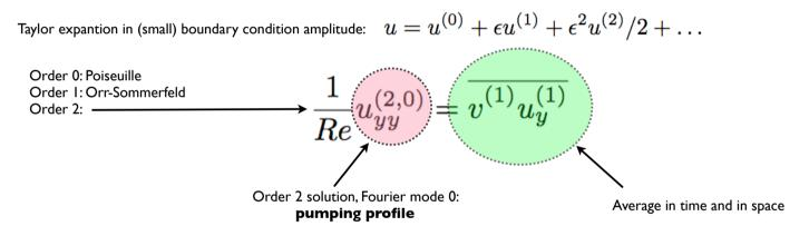
Order 0: Poiseuille - steady - due to the external pressure gradient Order 1: Orr-sommerfeld, oscillatory, no mean motion Order 2: Forced by the order one: pumping
