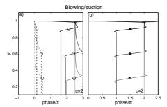
FIGURE 9. a) Phase of  $\hat{u}_y$  (plain)  $\hat{v}$  (broken) and b) departure from quadrature: phase  $(\hat{u}_y)$  – phase  $(\hat{v})$  –  $\pi/2$ , at  $Re_c=10^6$  for c=2 (light gray), and for wavespeeds such that the critical layers are at  $y_{cl}=0.3,0.6,0.9$  (from gray to black). The position of the critical layer is shown with the symbols.
