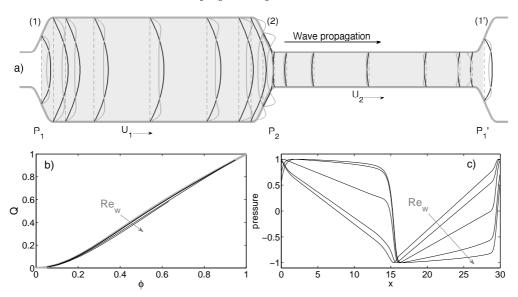
FIGURE 2. Configuration of the peristaltic pumping model (2.6). a) Velocity profiles for  $\phi = 0.5$ , wavelength L = 30 and  $Re_w = 1$  (black) and  $Re_w = 1000$  (light gray). For  $Re_w = 0.1, 1, 10, 100, 1000$ : b) the flux Q as a function of the constriction  $\phi$ , and c) the centerline pressure along one wavelength, normalized to the amplitude range [-1, 1].
