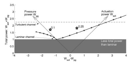
FIGURE 8. An alternative representation of the "power plane". Here the axes are rotated such that horizontal lines correspond to constant total power  $W_{act} + W_{pg}$ . The dotted line represents the power balance for blowing and suction for a fixed flux Q, at  $Re_w = Re_c = 2000$ . The two stars are the turbulent control results of Min *et al.* (2006) with wave amplitude 0.1 and 0.25.
