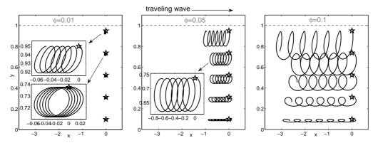
FIGURE 5. Trajectories of five particles at  $Re_w = 100, L = 10$  for 6 periods, with three wave amplitudes  $\phi = 0.01, 0.05, 0.1$ . Stars locate the particles initial position. The motion of flow particles is shown in the movies available with the online version of this paper.
