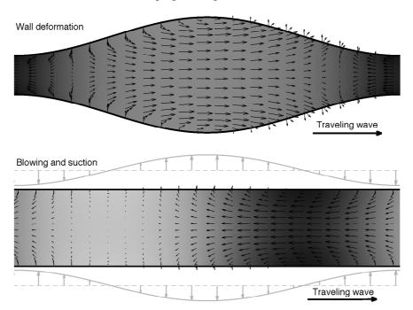
FIGURE 1. Velocity and pressure fields in the peristals is and blowing/suction cases, the Reynolds number is 300, wave amplitude is  $\phi=0.5$ , and the wavelength is L=6. The pressure field is indicated by gray shading: lowest pressure is black. The flow motion is best viewed from the movies available with the online version of this paper.
