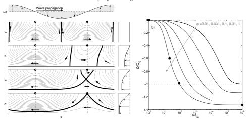
FIGURE 4. Traveling wave of blowing and suction. a) Instantaneous streamlines and averaged streamwise profile in the upper half of the channel for  $\phi=1$  at Reynolds corresponding to the black dots of b). b) Mean flux normalized by  $|Q_0|$  as a function of the Reynolds number for 5 different  $\phi$ .
