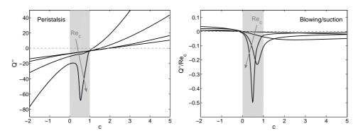
FIGURE 10. Wall actuation interaction with base flow: pumping flux as a function of the wavespeed c for  $Re_c = 1, 10, 100, 1000$ . The parameter range where a critical layer is present  $c \in [0, 1]$  is highlighted by a shaded strip.
