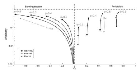
FIGURE 6. Flux and efficiency of pumping while varying the Reynolds number  $Re_w \in [1, 1000]$  (solid line), and the actuation amplitude  $\phi$ , for  $L = 2\pi$ . Note that the case  $Re_w = 1$  is not represented by an additional symbol.
