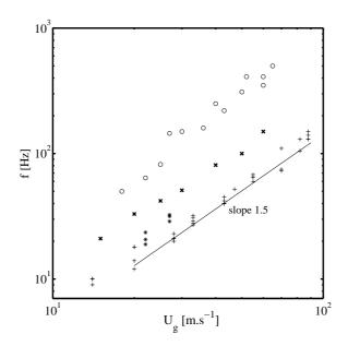
Figure 1: Experimental frequency vs. gas velocity for various sets of experiments with M > 4. (+) Data obtained by Raynal (1997) M = [4.2 : 2115], ( $\circ$ ) Marmottant & Villermaux (2004) M = [4 : 108], (x) Ben Rayana (2007) M = 16 and (\*) Matas *et al.* (2011) M = [5 : 14]. The most unstable frequency is shown to scale as  $U_g^{3/2}$  for large M.
