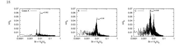
Figure 16: Simulation results. FFT of the position of the interface at x/e = 8 and M=20, r = 10.  $e/\delta_g = 0.5, 1, 2$  (from left to right). The forcing frequencies are not visible. The peak observed in the spectrum is more noisy for large  $e/\delta_g$  ratios.
