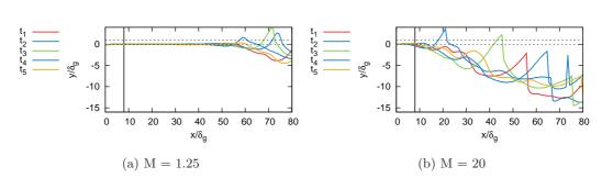
Figure 9: Interface position sampled at different times during one cycle ( $\Delta t^* = 3750$ ) The axis have been stretched to facilitate the visualization. The vertical line represents the location where the interface is sampled to obtain the FFT.
