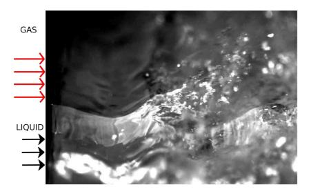
Figure 3: Visualization of the shear instability with both a laser slice and white light:  $U_q = 25 \text{ m/s}$  and  $U_l = 0.55 \text{ m/s}$ . e = 0.2 mm.
