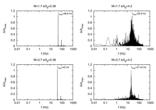
Figure 22: Experimental results in air/water conditions. FFT of the position of the interface for  $e/\delta_g = 0.38, 4.2$  and dynamic pressure ratio 1.7 and 3.7.  $U_g = 20$  m/s. When  $e < \delta_g$  a clear peak appears in the spectrum. The spectrum becomes broad and noisy for  $e > \delta_g$ .
