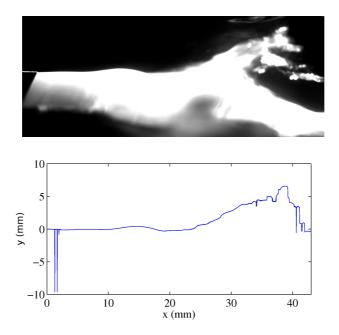
Figure 5: Top: Laser slice of the flow seeded with fluorescein. Bottom: interface location computed from the image:  $U_g = 20$  m/s and  $U_l = 0.70$  m/s. e = 0.2 mm.
