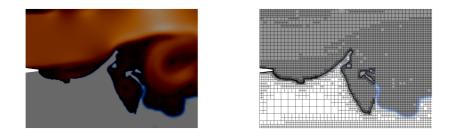
Figure 19: Zoomed view in the region near the splitter plate. Left: Velocity field (same color scale as in Figure 18). Right: Spatial mesh distribution.
