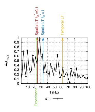
Figure 20: Fourier analysis of the interface height temporal evolution at  $x/\delta_g = 11$  obtained from numerical simulation, experiments and theoretical predictions by a temporal analysis and spatiotemporal analysis. Conditions of table 3.
