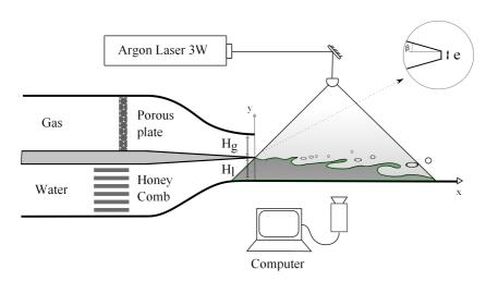
Figure 2: Sketch of the experimental set-up. Two splitter plates are used in the experiment: e = 0.2 mm and  $\beta = 4.15^{\circ}$ , and e = 2.2 mm and  $\beta = 4.1^{\circ}$ .
