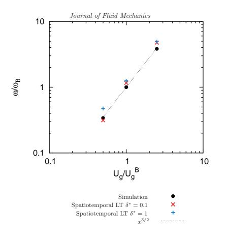
Figure 13: Peak frequency as a function of the gas velocity at large dynamic pressure ratios.  $U_g^B$  represents the gas velocity previously used to perform the simulations at constant gas velocity (Table 1) and M = 20.  $\omega_B$  is the observed frequency at these conditions.
