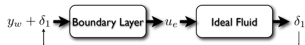
Figure 10: "Inverse method", the total geometry (boundary layer thickness and effective geometry) give the velocity which gives a total geometry, and so on.
