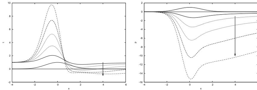
Figure 9: Non linear computation, left, the skin friction over a bump, the pressure over the same bump  $\alpha e^{-(2x/3)^2}$  for  $\alpha = 1, 2, 3, 4, 5$ . Notice that the skin friction becomes negative indicating a reverse flow on the lee side of the bump. In the separated bulb, the pressure is nearly linear.
