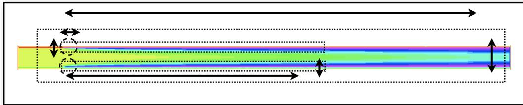
Figure 1: The Poiseuille flow in a pipe at temperature  $T_0$  in  $x < 0$  is experiencing a temperature discontinuity in  $x > 0$  to  $T_w$ . Iso temperatures are presented. This example contains several distinct scales near the discontinuity, near the walls, etc.
