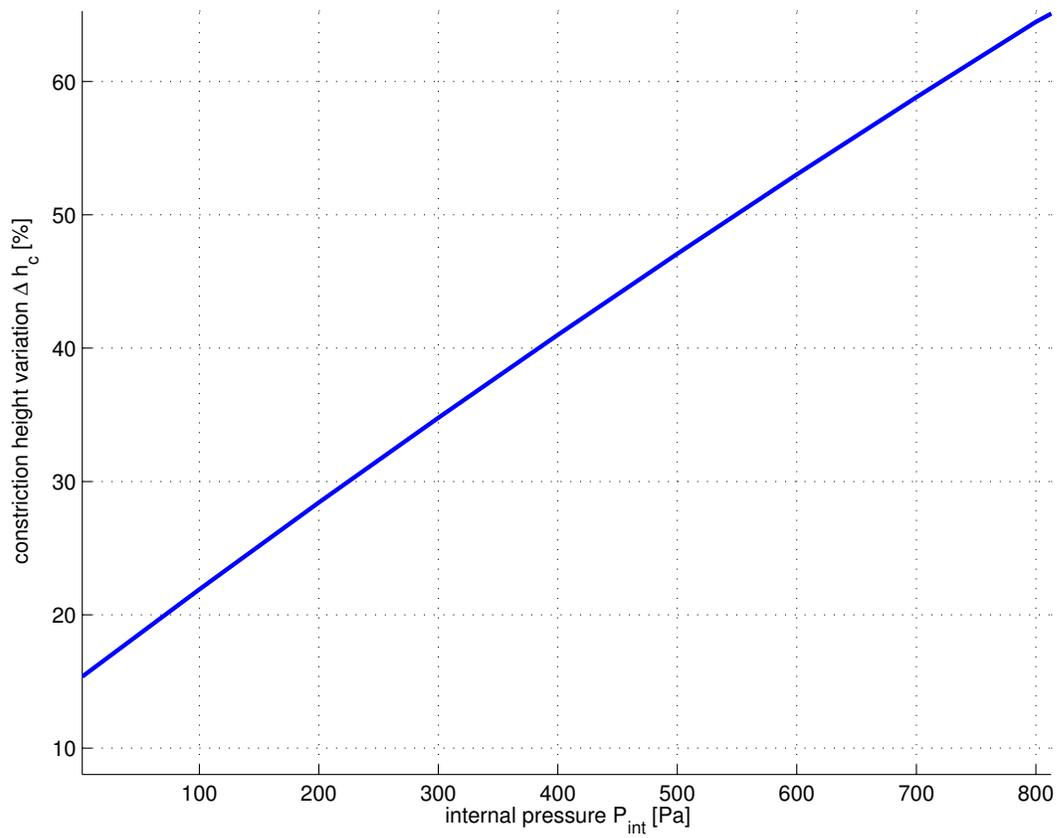
**Fig. 13.** Influence of the internal pressure  $P_{int}$  on the partial closure of the channel. Simulations with parameters :  $\Delta P = 150$  Pa,  $h_c = 1.5$  mm,  $E = 1.6$  MPa.
