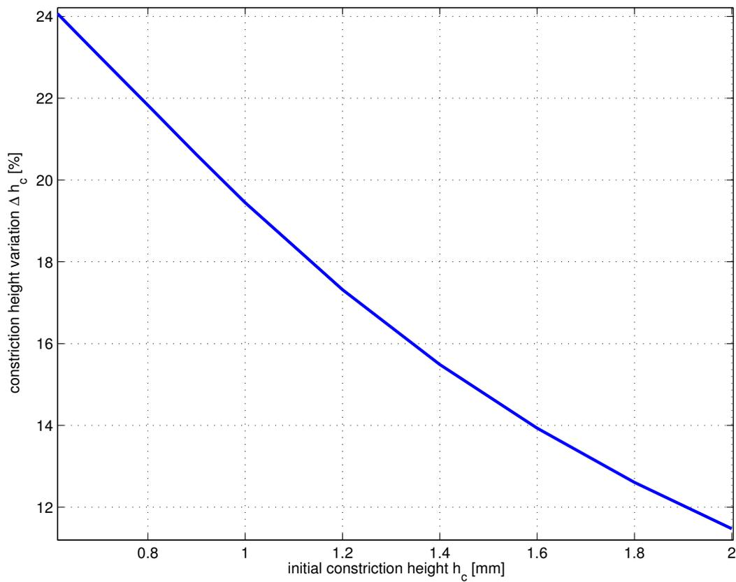
**Fig. 11.** Influence of the initial constriction height  $h_c$  on the partial closure of the channel. Simulations with parameters :  $\Delta P = 150$  Pa,  $P_{int} = 200$  Pa,  $E = 1.6$  MPa.
