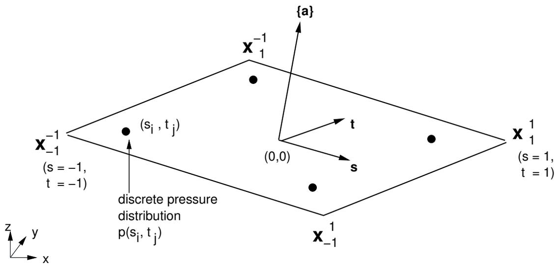
Fig. 4. Standard coordinate system associated to an element (e).
