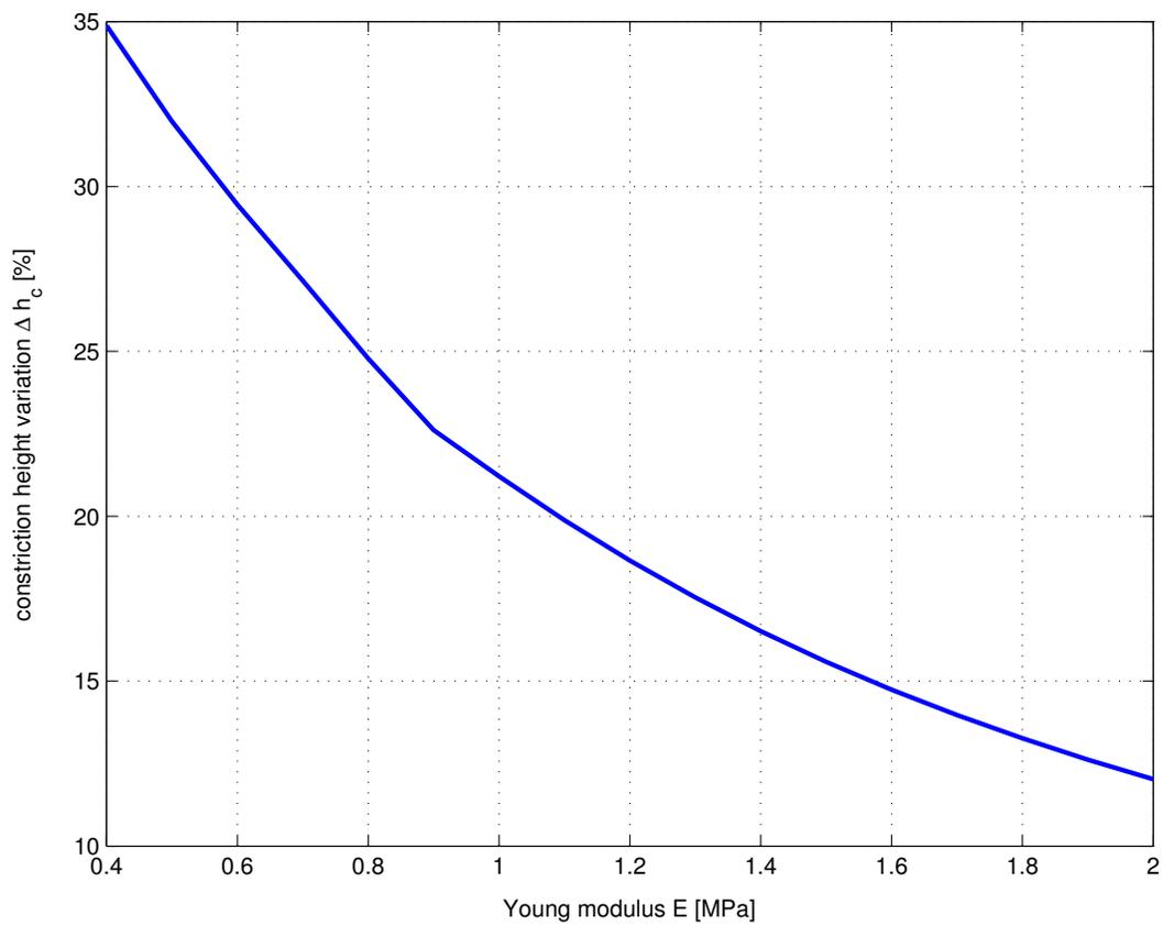
**Fig. 12.** Influence of the Young modulus  $E$  on the partial closure of the channel. Simulations with parameters :  $\Delta P = 150 \text{ Pa}$ ,  $P_{int} = 200 \text{ Pa}$ ,  $h_c = 1.5 \text{ mm}$ .
