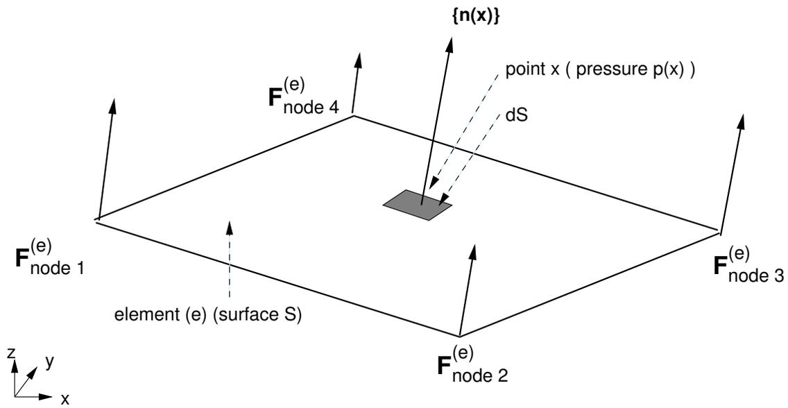
**Fig. 3.** Pressure and equivalent nodal forces on an element (e).  $\{\mathbf{F}_{\text{nodes}}^{(e)}\}$  is constituted of  $\mathbf{F}_{\text{node 1}}^{(e)}$ ,  $\mathbf{F}_{\text{node 2}}^{(e)}$ ,  $\mathbf{F}_{\text{node 3}}^{(e)}$ ,  $\mathbf{F}_{\text{node 4}}^{(e)}$ .
