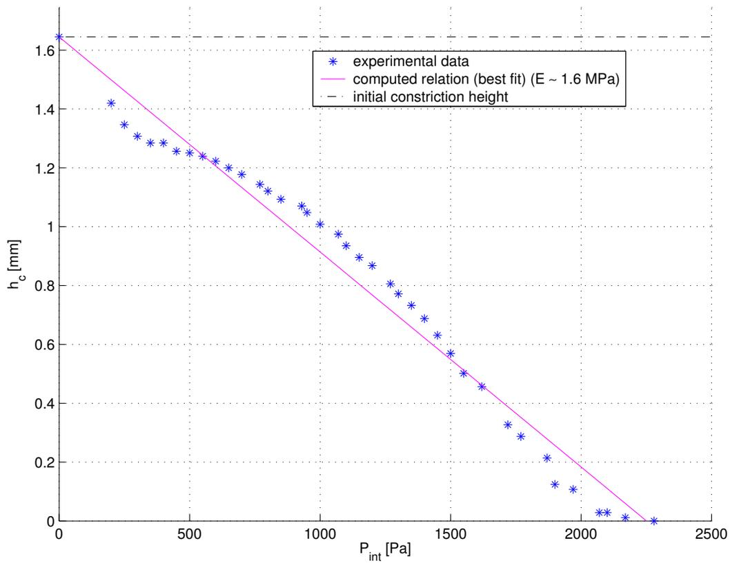
Fig. 8. Variations of the constriction height  $h_c$  in response to variations of the internal pressure  $P_{int}$ .
