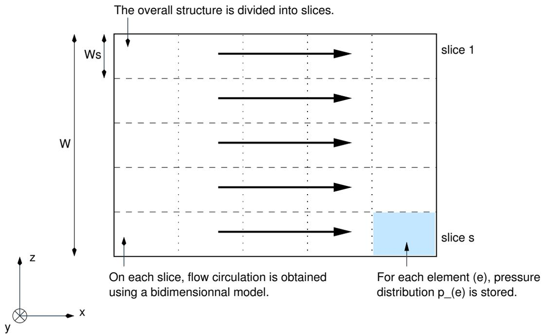
**Fig. 2.** Division of the structural model into slices for flow computation.
