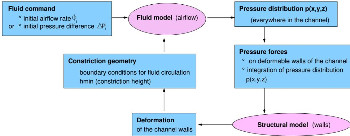
**Fig. 5.** *The general algorithm used for coupling fluid and structure.*
