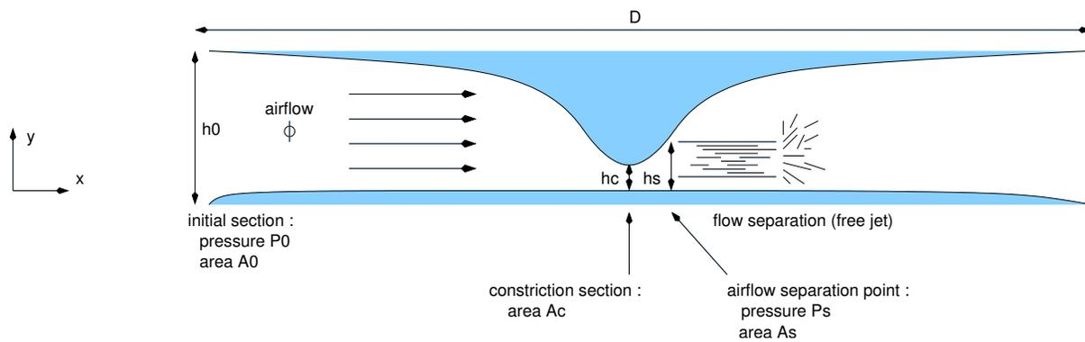
**Fig. 1.** *Flow inside a constriction.*
