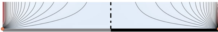
FIGURE 21. (Colour online) Left: isolines for the radial velocity \tilde{u}_r , extracted from the numerical simulations. Right: theoretical isolines for the radial velocity given by the composite expansion \tilde{u}_r^{comp} . Note that the transverse scale has here been stretched to visualize the boundary layer.
