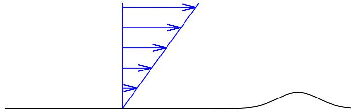
Shear flow over a topography  $f(x, t)$  at small Reynolds number
