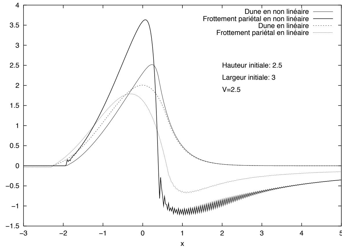
Abbildung 2: Comparing the skin friction perturbation ( $\tau - 1$ ) and the "dunes" in the linear and non linear cases
