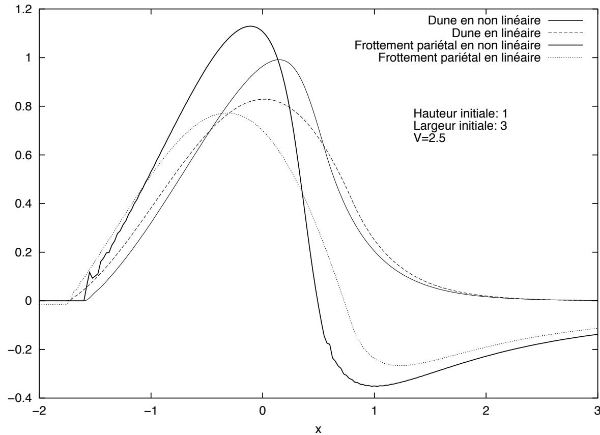
Abbildung 1: Comparing the skin friction perturbation ( $\tau - 1$ ) and the "dunes" in the linear and non linear cases, here with separation
