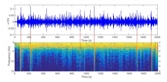
FIG. 9. Top: Temporal wave height signal for  $\tau=0.44$  ( $\epsilon_\eta=0.08$ ,  $\Delta f=0.16$  Hz). x=29.8 m. Bottom: Time-frequency spectrum  $S_\eta(f,t)$  of the corresponding wave height  $\eta(t)$ . The color bar is a logarithmic scale of the spectrum amplitude. Large amplitude events of the wave signal correspond to maxima of the spectrum at high frequencies (see solid lines).
