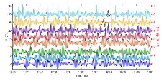
FIG. 3. Experimental evolution along the basin length x of the wave height  $\eta(t)$  recorded at different probe locations (from bottom to top: x=0, 3.4, 7, 12.6, 16.3, 20.1, 24.9, and 29.8 m).  $\tau=0.44$  ( $\epsilon_{\eta}=0.08$  and  $\Delta f=0.16$  Hz). Dashed (red) lines have a slope corresponding to the group velocity  $c_g$ . The dashed (black) line on top of the two upper curves is the theoretical shape of the envelope soliton of Eq. (8).
