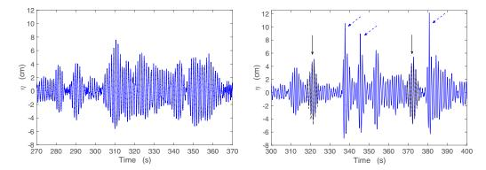
FIG. 7. Left: Wave height signal recorded close to the wavemaker at the first probe (x = 3.4 m).  $\tau = 0.55$  ( $\epsilon_{\eta} = 0.1$ ,  $\Delta f = 0.16$  Hz). Right: Same part of the signal recorded at the last probe (x = 29.8 m) showing coexistence of two envelope solitons (see full arrows) and three extreme events (see dashed arrows). (- - -) Theoretical shape of the soliton from Eq. (8).
