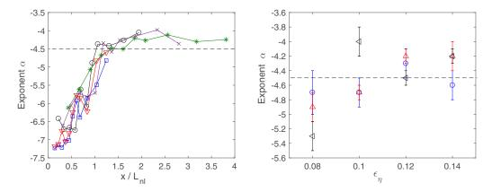
FIG. 11. Left: Exponent  $\alpha$  of the wave spectrum in  $f^{\alpha}$  as a function of dimensionless distance  $x/L_{nl}$  for different ratios  $\tau$  (same symbols as in Fig. 5). Right: Exponent  $\alpha$  as a function of the wave steepness for different modulation bandwidths  $\Delta f = 0.09$  ( $\circ$ ), 0.16 ( $\Delta$ ), 0.24 ( $\lhd$ ) Hz at  $x/L_{nl} > 1.2$ . Dashed lines show the 1D wave turbulent prediction -9/2.
