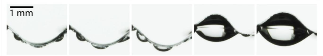
PDMS strip made hydrophilic on lower face experiment lasts ~ 3 min
