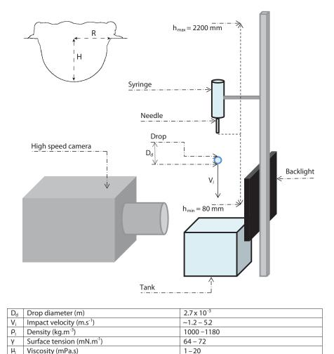
FIG. 1. Schematic view of the experiment and the values of the main physical parameters used. In the top left corner is a schematic of the cavity, defining the depth H and radius R of the cavity.
