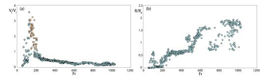
FIG. 4. (a) The jet velocity normalized by the drop impact velocity and (b) the top drop radius normalized by the impacting drop radius, following a drop impact on a free surface of water, as a function of the Froude number:  $Fr = V_i^2/gD_d$ . The yellow circles indicate that the jet is accompanied by a bubble entrapment.
