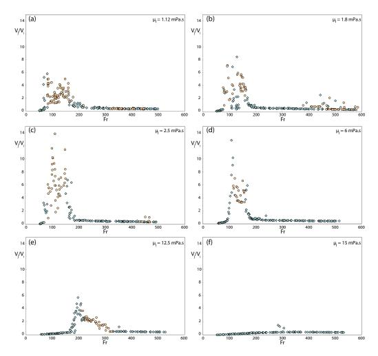
FIG. 5. Jet velocity  $V_J$  normalized by the drop impact velocity  $V_i$ , following a drop impact on the free surface of viscous liquid with six different viscosities  $\mu$ , as a function of the Froude number:  $\text{Fr} = V_i^2/gD_d$ . The yellow circles indicate that the jet is accompanied by a bubble entrapment.
