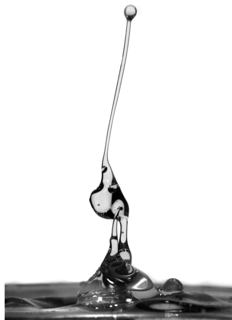
FIG. 2. Snapshot of a 15 cm high jet springing up above the free surface (Ref. 1) for an airflow rate of 3.5 \text{ l}\cdot\text{min}^{-1} .
