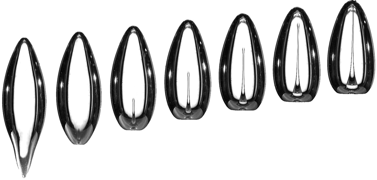
FIG. 1. Time sequence of the jet developing inside a large bubble just after its release from a submerged nozzle. The large bubble pinches off at the first image and the back-to-equilibrium dynamics exhibits an intense and concentrated jet. The time lapse between the snapshots is \Delta t = 3 ms. The entire sequence lasts 18 ms and the bubble height, right after detachment, is H = 4.22 cm. The bubble front velocity is V_{\text{front}} = 0.67 \text{ m} \cdot \text{s}^{-1} and the jet velocity is V_{\text{jet}} = 2.69 \text{ m} \cdot \text{s}^{-1} . The liquid viscosity is \mu = 420 \text{ mPa} \cdot \text{s} . The gas is injected through an injector of diameter d = 1.8 \text{ mm} at an airflow rate of Q = 4.4 \text{ l} \cdot \text{min}^{-1} . The fluid height is h = 10 \text{ cm} .
