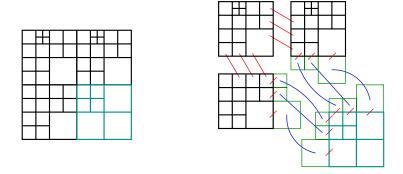
Figure 2. Sketch of parallel domain decomposition on two processors within Gerris. Left: leaf cells colored according to processor number. Right: corresponding structure. The four quadtrees making up the domain are shown, together with "stitches" (red), ghost cells (green), and parallel boundary conditions (blue).
