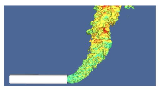
Figure 12. Three dimensional representation of the water/oil interface of a plume generated by the oil leak. Fr = 10. In colors, the norm of the vertical velocity at the interface. The AMR techniques implemented in Gerris allow capturing the small structures generated by the turbulence of the flow at the tube exit while keeping a relatively low total number of nodes in all the computational domain when compared with an uniform mesh.
