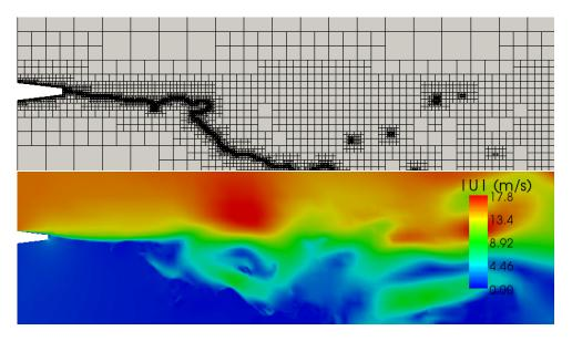
Figure 11. Adaptive mesh (top) and velocity field (modulus) of the flow near the injector. The mesh is adapted at the interface for an accurate representation of the interface. The important velocity gradients induced in the gas phase are also accurately captured by applying dynamically adaptive criteria.
