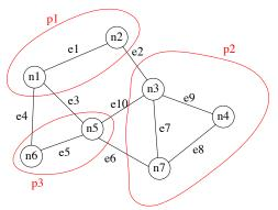
Figure 3. Example of graph partitioning. Nodes and edges can have an associated weight. The subgraphs p1, p2, p3 are a partition of the initial graph. The goal is to obtain a balanced partition (each subgraphs have comparable total weight) while minimising the number (or total weight) of edges cut.
